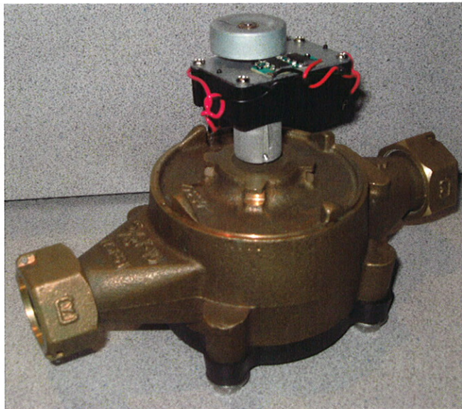
Figure 6: DC Generator Mounted on the Modified Water Meter
